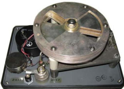
The remarkable thing is that after some 70 years, the device is still quite useful for measuring antenna patterns. Although it is not particularly sensitive it may be used for both 2 m, 70 cm amateur and
