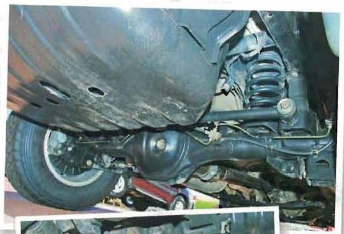
The low-slung transfer is protected by a sturdy crossmember, but it decreases ramp-over angle and clearance significantly. The Jackaroos are still capable in the rough, but more suited to touring duties
