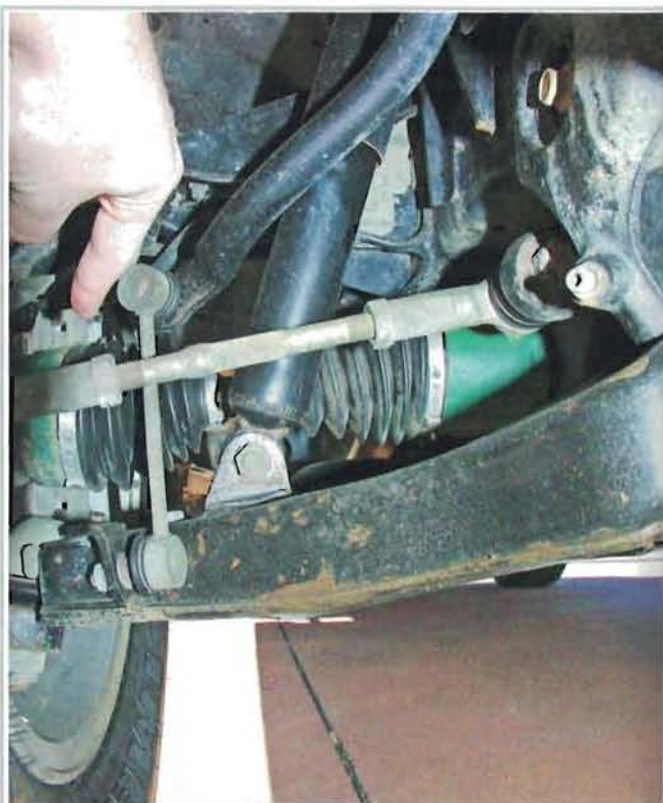
The tie rod ends and CV shafts do wear over time, but are easily replaced. The later auto-locking hub models tend to chew out CVs, as do vehicles lifted more than a couple of inches. Pay special attention to these models
