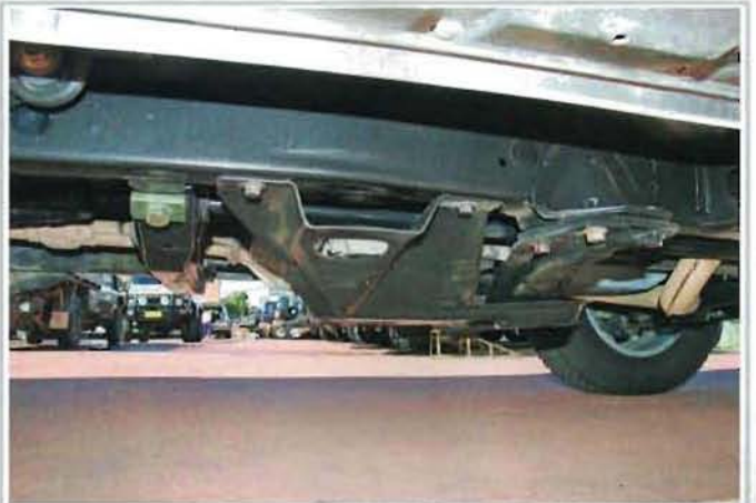
The low-slung transfer is protected by a sturdy crossmember, but it decreases ramp-over angle and clearance significantly. The Jackaroos are still capable in the rough, but more suited to touring duties
